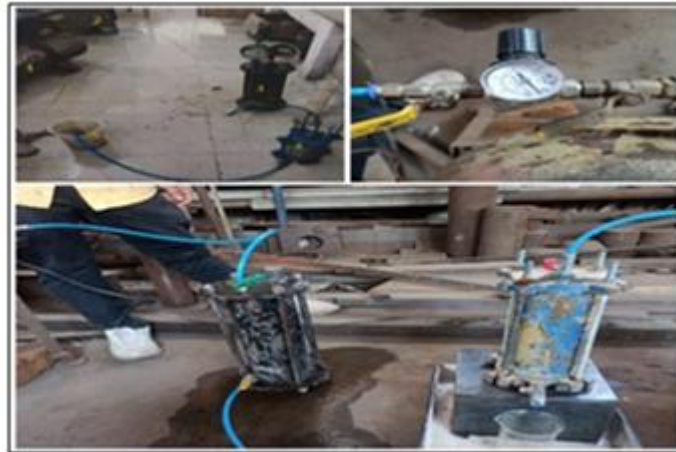
Figure 7. Adherent washout strength
