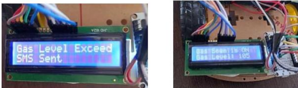
Fig.7.2 Gas Leakage Level-High
