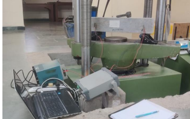
Figure 4: Flexural Testing of Beam.
