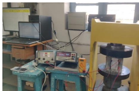
Figure 3: Compressive testing of cube
