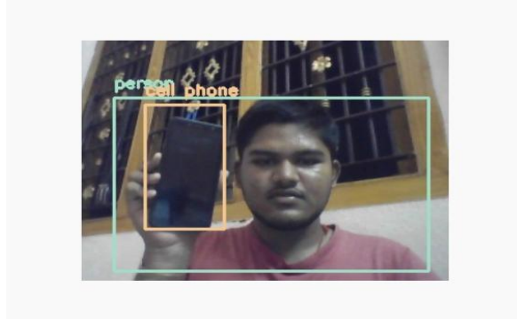
Fig 8. An image is taken by the user holding a cell phone where the yolo_v3 detects the two objects and prompts a voice message as person, cell phone
