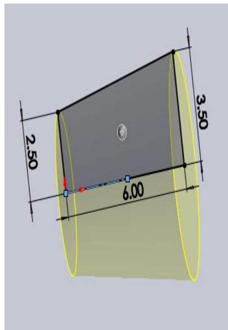
**Figure 0.4 Blunt Shaped Control Valve with Minor Dia 2.5 Mm & Major Dia 3.5 Mm**
