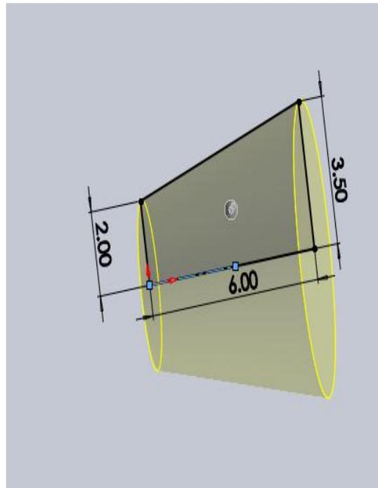
**Figure 0.3 Blunt Shaped Control Valve with Minor Dia 2 Mm & Major Dia 3.5 Mm**
