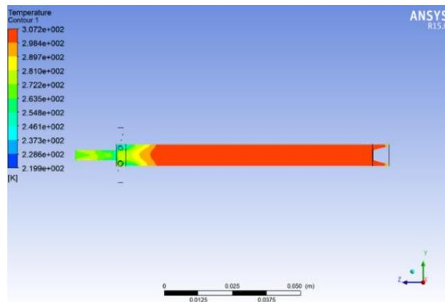
Figure 0.5 Temperature Contour- Inlet Nozzle 10 Mm Length
