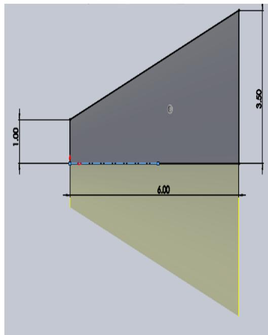
Figure 0.2 Blunt Control Valve with Minor Dia 1 Mm & Major Dia 3.5 Mm
