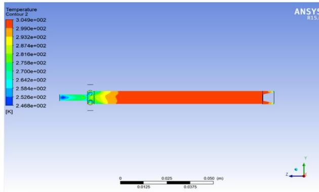
Figure 0.4 Temperature Contour- Inlet Nozzle 8 Mm Length
