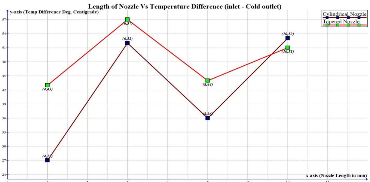
The graph 6-3 shows the results for temperature difference which results in better temperature drop and for inlet nozzle length of 6 mm for taper nozzle and 10 mm length for cylindrical nozzle.
