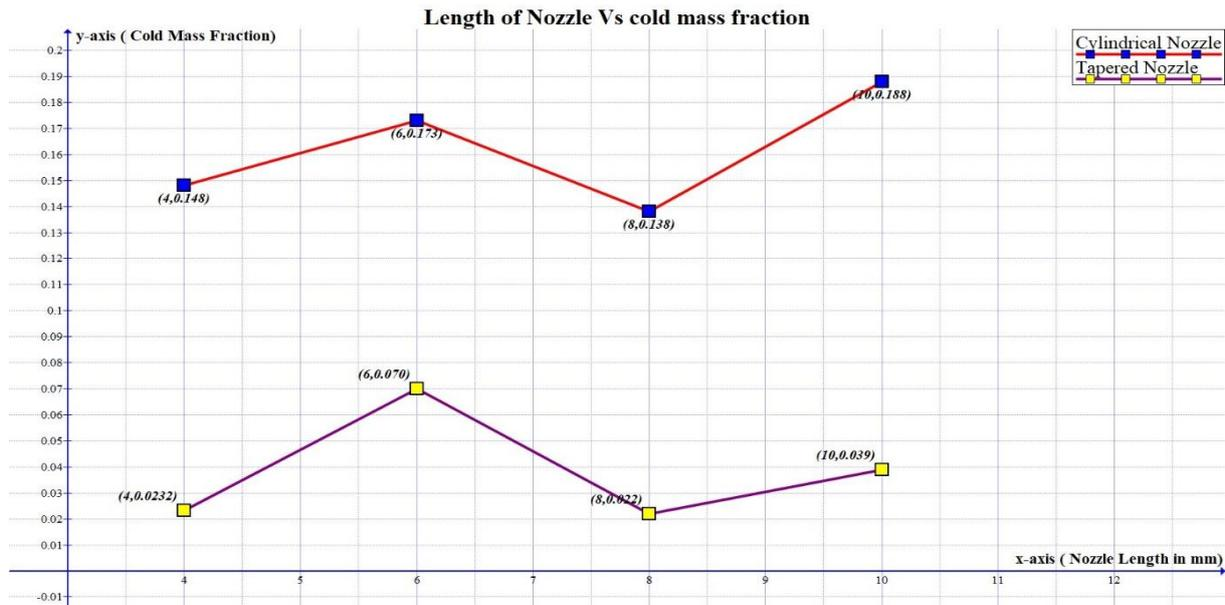
The graph 6-4 shows the results for cold mass fraction which results in better cold mass fraction and for inlet nozzle length of 10 mm for cylindrical nozzle and 6 mm length for cylindrical nozzle.
