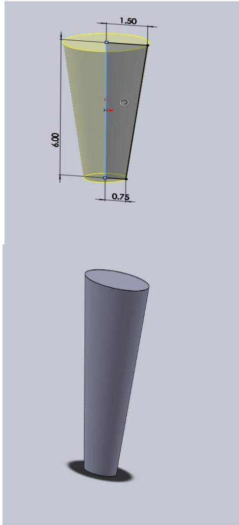
Figure 0.1 Tapered Inlet Nozzles
