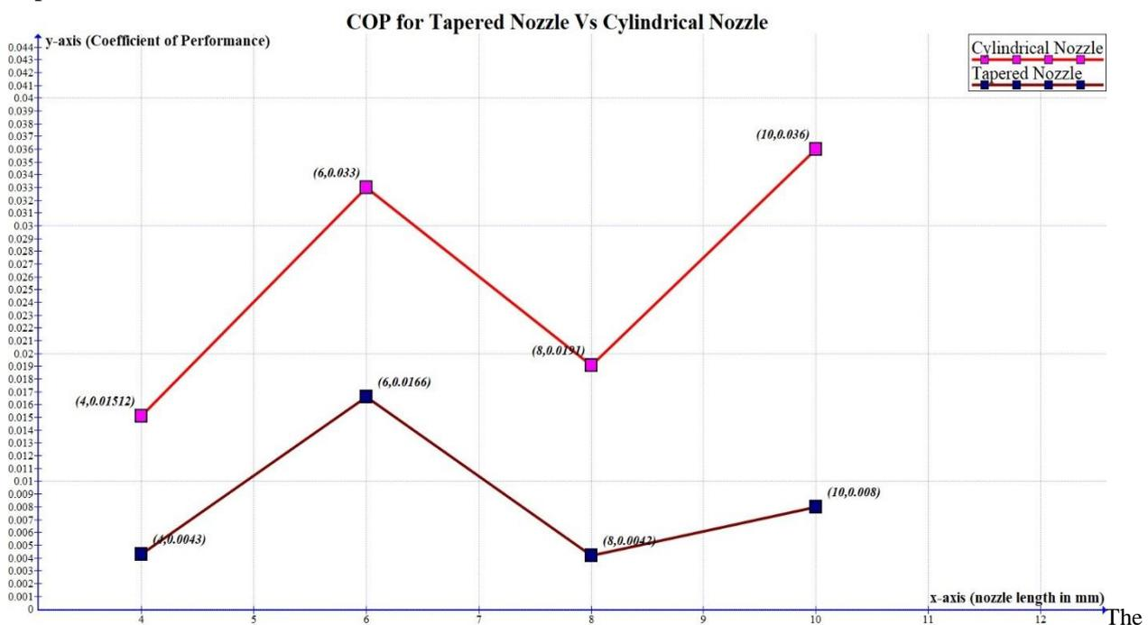
Graph6-1 shows the results for coefficient of performance which results in better coefficient of performance and cold mass fraction for inlet nozzle length of 10 mm for taper nozzle and 6 mm length for cylindrical nozzle.
