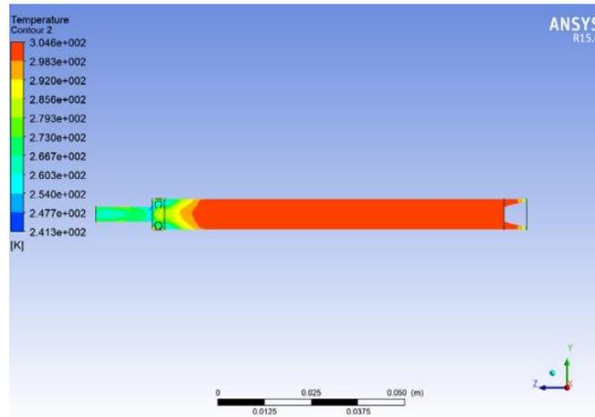
Figure 0.1 Temperature Contour- Inlet Nozzle 4 Mm Length
