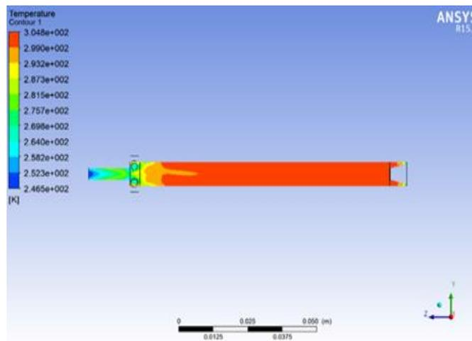
Figure 0.2 Temperature Contour - Inlet Nozzle 6 Mm Length
