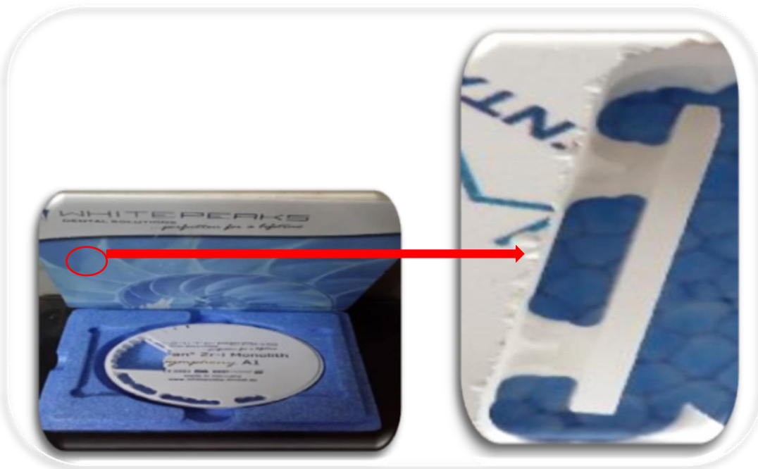
Figure 1: The attached pre-sintered specimen after milled from the zirconia blank.
