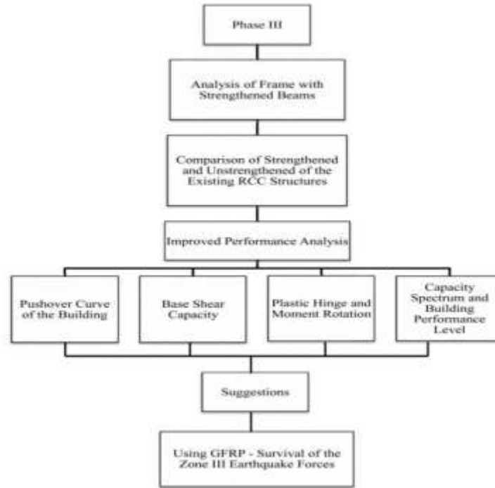
Figure 3: Analysis of Bare Frame with Strengthened Beams
