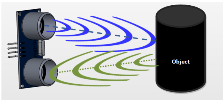
Fig.8 Working Of Ultrasonic Sensor
