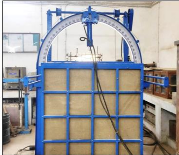
Figure 3 Model foundation tank
