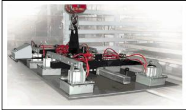
Fig 5. Schematic representation of magnetic gripper[26]
