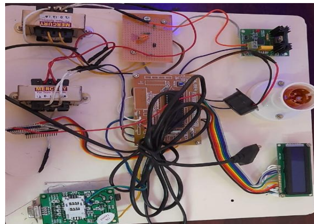
Fig 2: Hardware of smart energy meter
