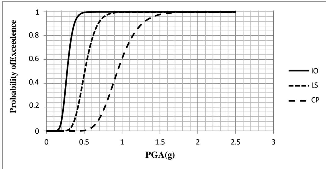
Figure 4.2 Fragility curve using Cornell's Method
