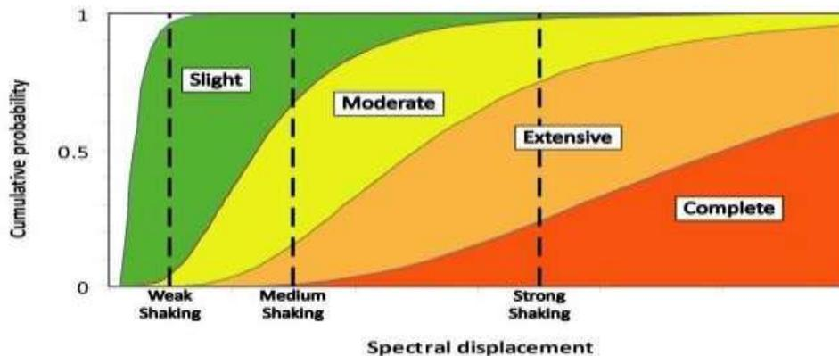
**Figure 1.3 Fragility curves for 4 different limit states(TobasandLobo 2008)**
