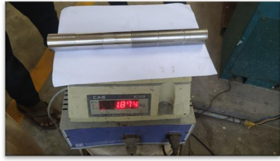
Figure 3.3. Weighing workpiece after machining
