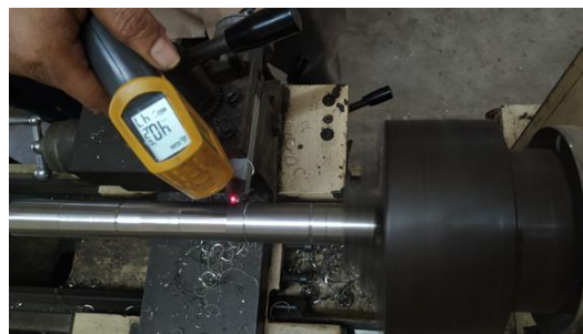
Figure 3.6. Measuring tool tip temperature while machining
