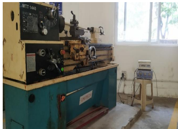
Figure 3.1. Centre Lathe with digital weighing machine
