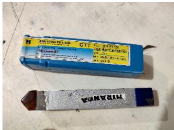
Figure 2.2. Tungsten Carbide Tipped Tool
