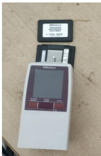
Figure 3.4. Talysurf Surface Roughness Tester
