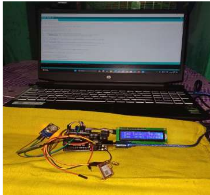
(WORKING MODULE OF GAS DETECTION SYSTEM)
