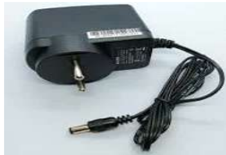
(12V CHARGER FOR POWER SUPPLY)
