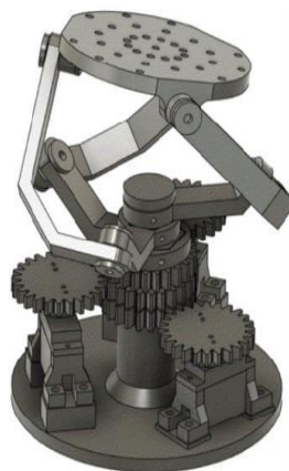
Figure: 1 Spherical Parallel Manipulator
