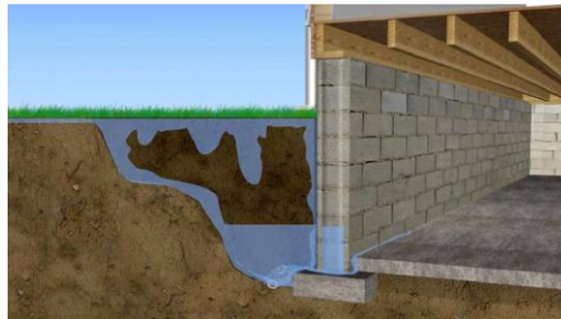
Fig 2 (Foundation damage due to Surface Water Infiltration)
