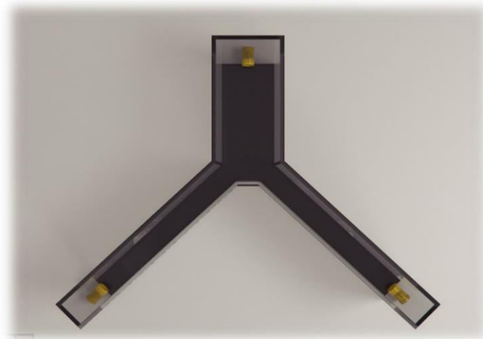
Figure 16. Zebrafish Y Maze Flow Modification: This Flow-Through Y-Maze is a modification of the Zebrafish Y-Maze. The flow-through Y-Maze apparatus consists of an aquatic tank shaped like a capital 'Y.' Two of the arms serve as the goal arms. The modification of the conventional aquatic Y Maze involves the addition of the pressure controlling flow meters at each intake valve of the goal arms to control and measure the rate of flow of the fluids into the arms. The Zebrafish Y-Maze is an adaptation of the rodent Y-Maze (also see T-Maze). The 'Y' design is preferred over the 'T' design due to its natural turns., Grella, S. L, Kapur, N., & Gerlai, R. (2010)
