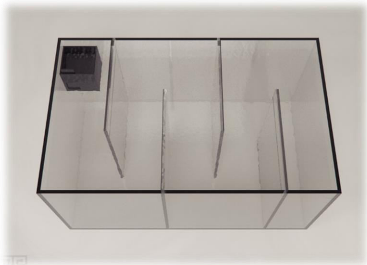
Figure 12 The Zebrafish Sociability Chamber is used for studying the exploration and socialization behaviors in zebrafish. The concept of zebrafish sociability chamber derives from the 3-chamber sociability device used for socialization testing in rodents. The 5-chamber sociability tank analyzes the socialization behavior in fish by allowing them to interact with the social stimuli and explore the tank. Araujo-Silva, Pinheiro-da-Silva, Silva, and Luchiari (2018)
