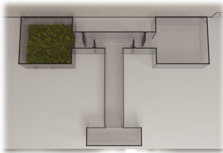
Figure 22. The Zebrafish Bifurcating T Maze has been described in the literature as a screening test for the role of nicotinic acetylcholine receptors in Zebrafish. It has been traditionally used as a screening maze, but can also be used for choice and learning experiments. Al-Imari, L., & Gerlai, R. (2008) be provided by the user. (Cognato, G., Bortolotto, J., Blazina, A., Christoff, R., Lara, D., Vianna, M., and Bonan, C., (2012)
