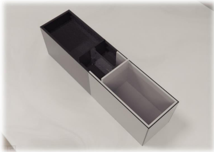
Figure 11. The Light Dark Tank for Zebrafish is an acrylic tank (15 cm × 10 cm × 45 cm height × width × length) that is divided equally into one-half black and one-half white. Walls and bottom are either black or white, so as to create a similar experimental paradigm to the rodent light dark box. The tank contains central sliding doors, colored with the same color of the aquarium side, thereby defining an uncolored central compartment measuring 15 cm × 10 cm. Bourin, M., & Hascoet, M (2003)
