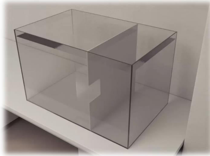
Figure 17. Zebrafish Environmental Enrichment Chamber: this is a widely used task to evaluate spatial and non-spatial learning as well as memory in zebrafish. The watertight apparatus is outlined by a dark panel; covering one side of each compartment as a visual cue to provide an axis of orientation for right/left discrimination. The apparatus is primarily used for learning and memory but can also be used for various toxicity experiments. Bergendahl I.A, Salvanes A.G.V, Victoria A. Braithwaitec V.A (2015)
