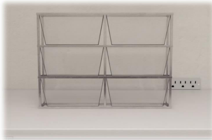
Figure 24. The Vertical Tank Array is used for anxiety experiments for Zebrafish. Vertical diving behavior is used to assess anxiety in zebrafish. Narrow tanks minimize horizontal movement to maximize the behavior assessment. Each tank holds 1.5L in a trapezoid pattern. Set of 6 arrays come together with a housing apparatus for easy video grading. Cachat, J.M. et al. and Kalueff, A.V. & Cachat, 2010).
