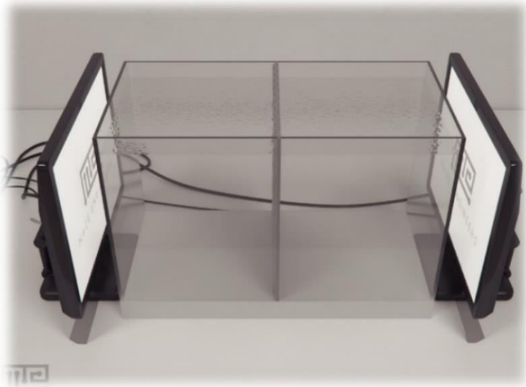
Figure 9. The Zebrafish Shuttle Box presents an automated method for high throughput learning paradigm testing. In this protocol, two screens are used from an automated computer screen to create computer animated zebrafish images, or any image in which the researcher specifies. This simple paradigm between binary choices makes this a useful high throughput assay for zebrafish. (Al-Imari, & Gerlai, 2008)
