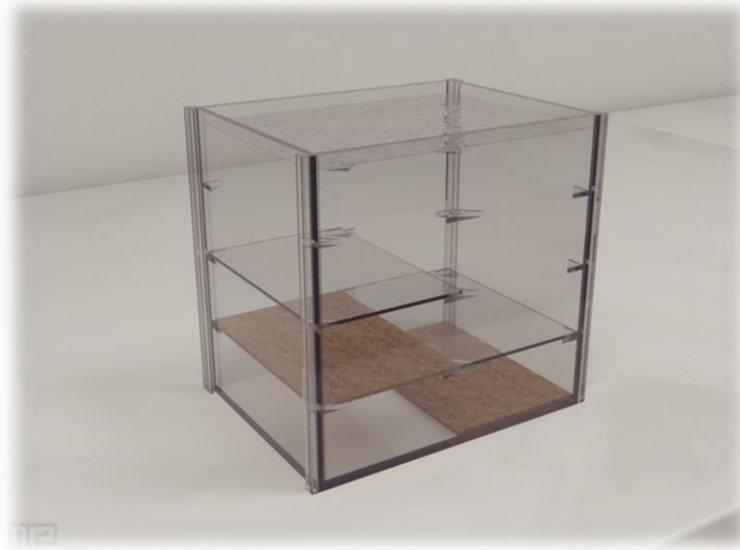
Figure 13. The Black white preference tank assesses for wall color stimuli on diving, and the effects of depth stimuli on scototaxis. The Black White preference tank allows for three separate configurations. The split-depth tank configuration is composed of one side of the tank that is set to a depth of 10cm using a partition while the other side is set to a depth of 15cm. In the shallow configuration, both sides can be set to a depth of 5cm. In the deep configuration, both sides of the tank can be set to 15cm. Gravel substrate is placed on a floor 5 cm below the plexiglas partition on each side. The sides of the tank are either left uncovered (transparent), covered in black paper (black), covered in white paper (white), or covered in black on one side, and white on the other. Rachel E. Blaser, R.E., & Rosemberg, D.B. (2012)
