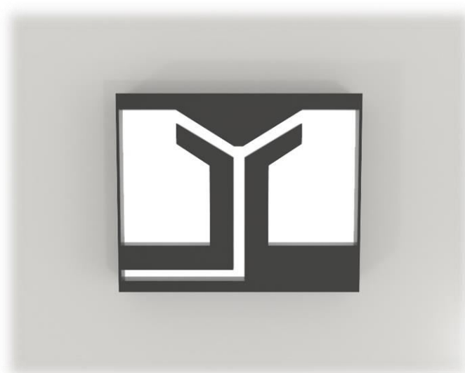
Figure 32. The Zebrafish larvae Y Maze takes advantage of a unique backlighting set-up to allow for fine behavior task assessment in larvae. Similar to the Zebrafish Larvae T apparatus and Drosophila mazes, this apparatus comes with a start lane, bidirectional swimming pools, and a unique backlight for easy video tracking. An easy-to-use cover seals the pools and watertight chambers ensures that you'll be able to use this apparatus for years to come. The apparatus comes with: Lid, Chambers, Backlight (Best, J. D., Berghmans, S., Hunt, J. J., Clarke, S. C., Fleming, A., Goldsmith, P. and Roach, A. G. (2008)
