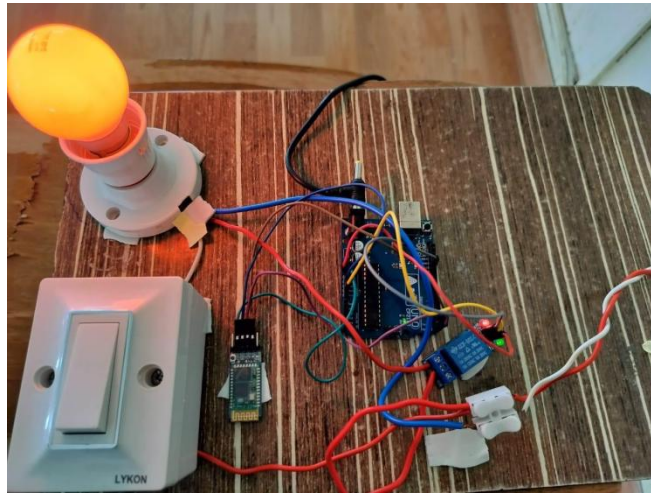
Fig 6.1: Smart Lighting system
