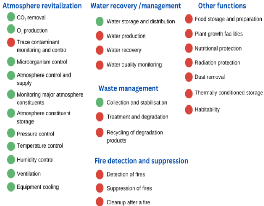
Fig: 5 Life support features as a function of mission length:1–12 hours. Credit: NASA
