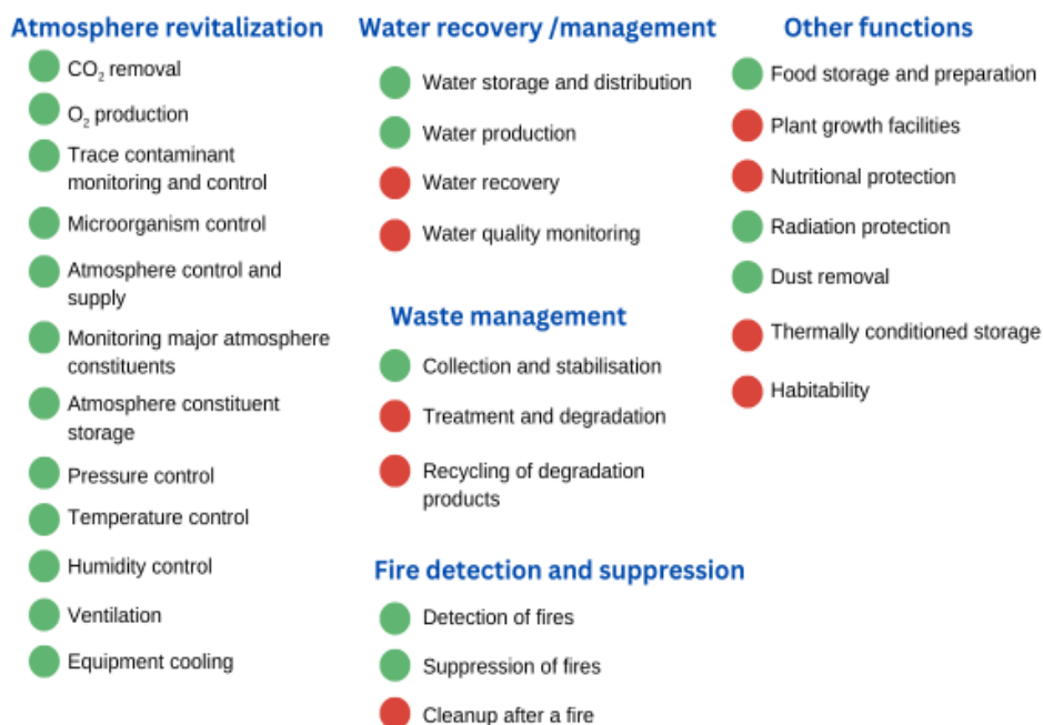
Fig: 6 Life support features as a function of mission length: 1–7 days. Credit: NASA
