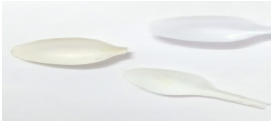
Fig:-shows single use PVC spoons as ceramic finger pad mould.
