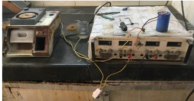
Fig. 8: Electrically controlled polishing on specimen(R.I.M.T., BAREILLY)
