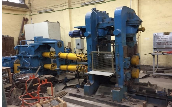
Fig. 5: Compaction of billet using Rolling mill(R.I.M.T., BAREILLY)
