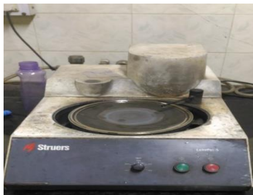
Fig.7: Mirror like Polishing using velvet (R.I.M.T., BAREILLY)
