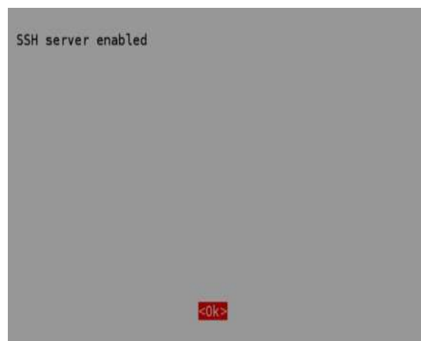
Figure 4.2 SSH server Enabled
