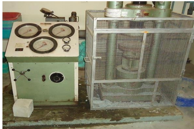
Figure 2: Test setup for compression
