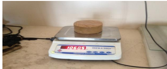
Fig 6: Weighing of specimen
