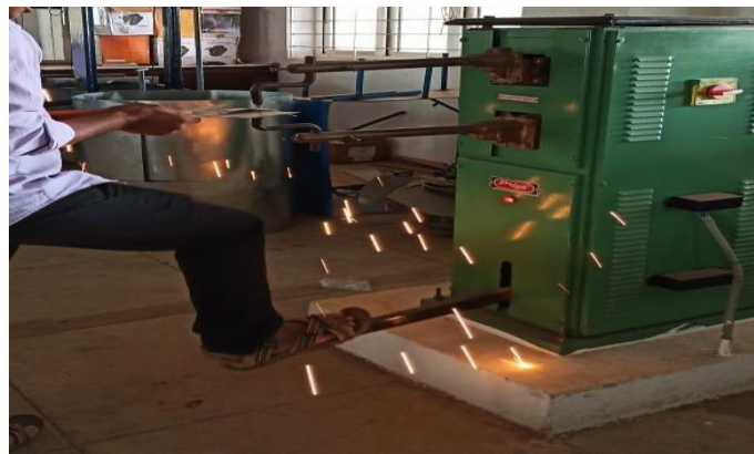
Fig:12 spot welding
