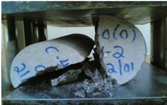
(a) Control concrete at failure
