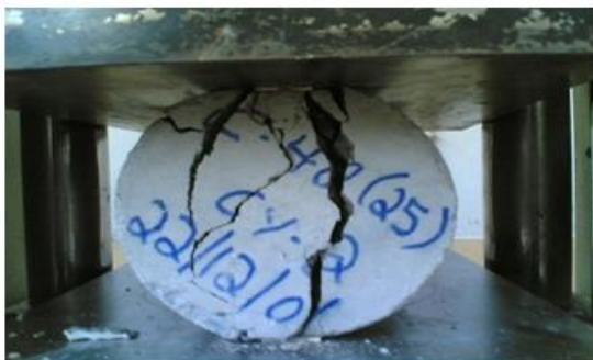
(c) Rubberized concrete at failure
