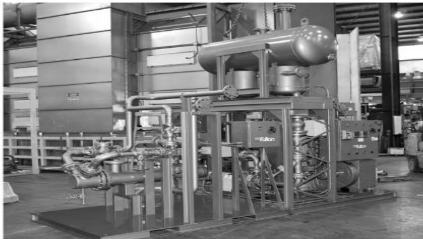
Figure 1: Thermal Fluid Heating System
