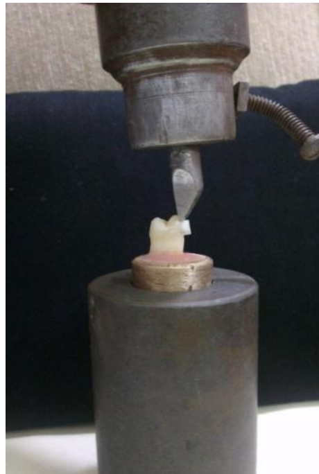
Figure (5): Knife-edge blade in a Universal Testing Machine was applied to the Base of cylinder
