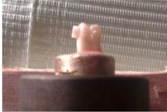
Figure (4): Cylinder of sealant adhering to the enamel surface
